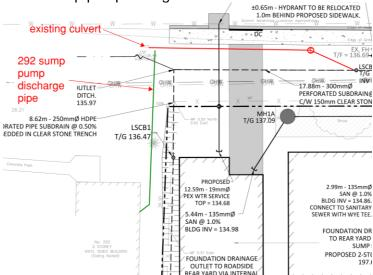
There is minimal cover on the proposed storm sewer within the Town's right-of-way
