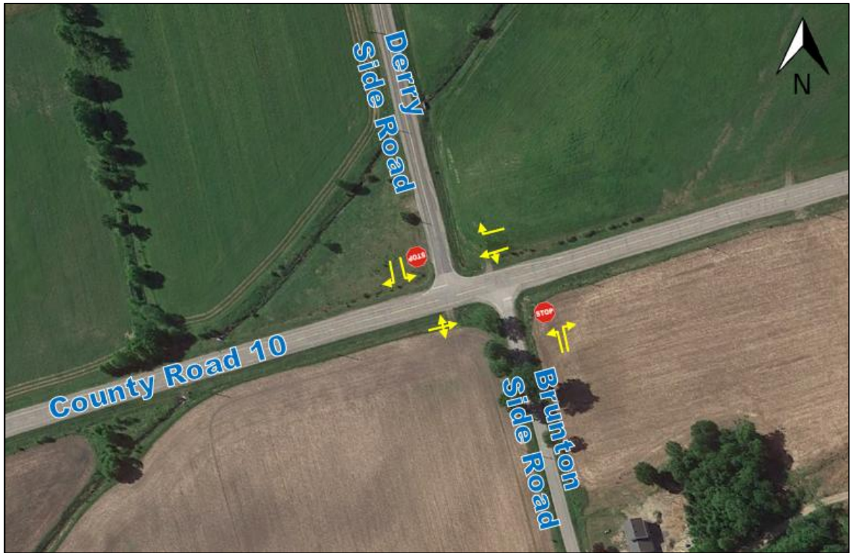
Figure 3-1. Existing Lane Configuration for Study Intersection
